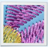
Invisible & Smart Secure Securing stitches become invisible as the tie-on/off stitches are sewn in stitch direction. Smart secure adds tie-on/off stitches to a design, if none are preset.
